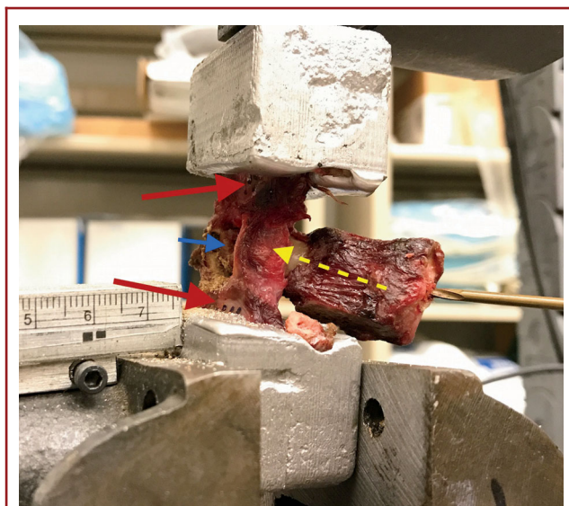
FIGURE 7. After cutting the C1 ring and applying 20 N preload with the odontoid (blue arrow) in place, the distance between the lateral masses (red arrows) was remeasured. Less than a millimeter and a half stretch in the TAL (yellow arrow) from baseline was noted.
