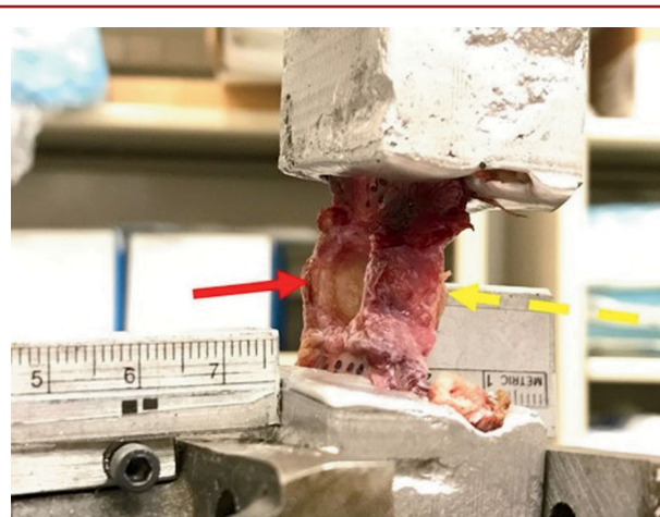
FIGURE 2. Baseline lateral mass distance was measured prior to disconnecting the anterior arch of C1 (red arrow) with the TAL (yellow arrow) maintained in its neutral zone.
